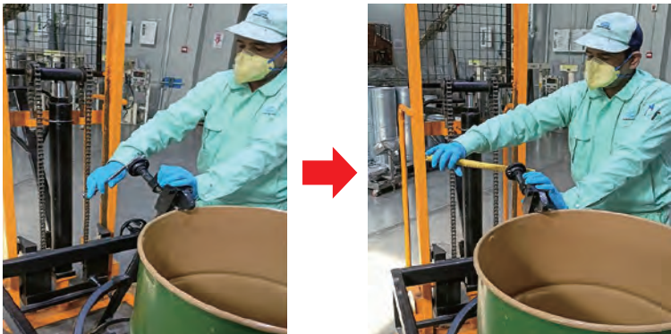
Before: A ring wrench was used After: A fixed handle has been attached
