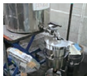
Half-closed lid to reduce exposure risk during product-filling work
