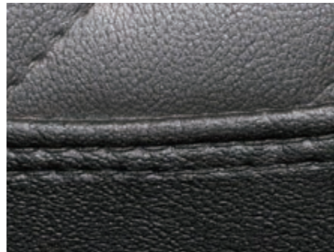
In-mold coating surface achieved using 458W
