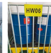
Palettes for preventing the leakage of coating waste
